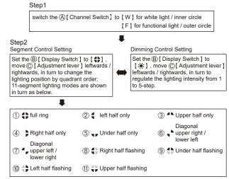
[Notice]: 1.  $\textcircled{3} \sim \textcircled{1}$  are on the mode of 1:2 brightness ratios, the blink indicates the brightness is lower.
